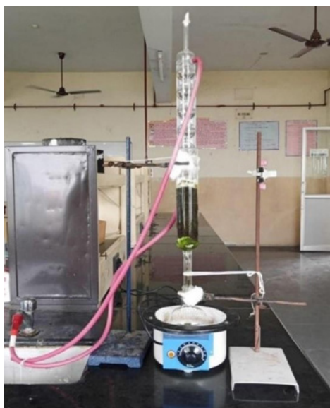
Figure 3: Working of Soxhlet apparatus 7
