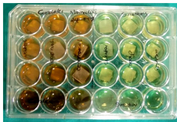
Figure 4: Inoculated acrylic chips in culture media for biofilm formation.
