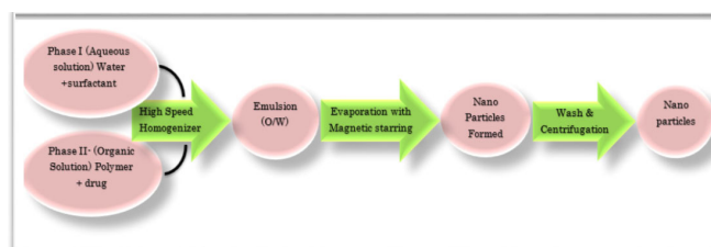
Figure 4: Schematic representation of the solvent evaporation method 27 .
