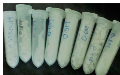
Figure 2: Powdered form of different concentration (0.1M to 0.8M) of ZnO nanoparticles in eppendorf.
