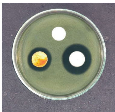
Figure 5: Scleral Resin Disks Immersed in Two Solutions Along with a Control Group Disk Propelled in SDA Plates inoculated with Candida Showing Zone of Inhibition.
