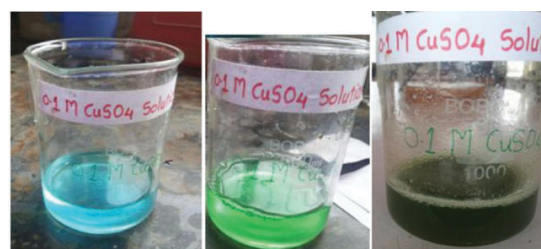
Figure 1c: 0.1 molar copper sulphate solution, d-Copper sulphate solution+Coriander leaves, e-CuNP settle at bottom.
