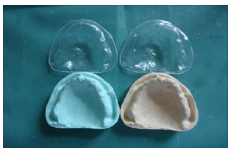
Figure 1: Denture Base models prepared with thermoplastic resin sheet of 2mm thickness using a vacuum forming machine.
