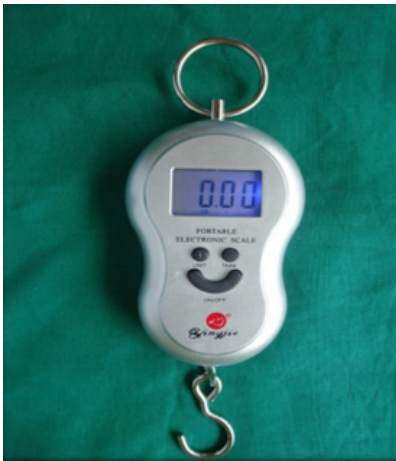
Figure 3: Electronic scale used to measure the load required to dislodge the denture bases.
