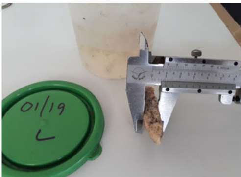
Figure 3: Measurement of Thickness.
