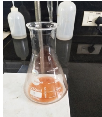
Figure 8: Formation of brown precipitate in treated wastewater.
