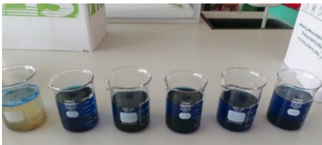
Figure 7: Presence of brownish precipitate in treated wastewater.
