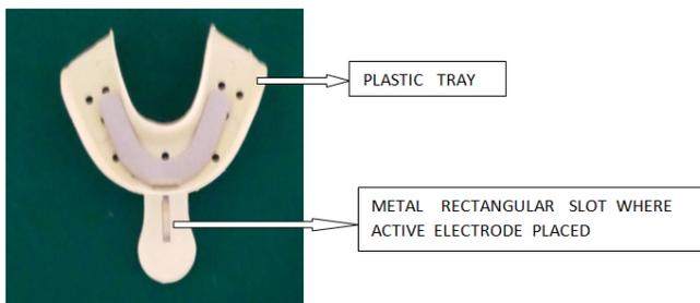
Figure 3: Parts of plastic tray.
