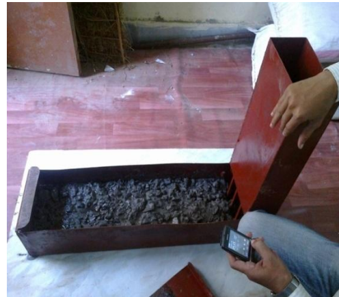
Figure 4: L-Box test apparatus used
