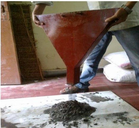
Figure 3: V-Funnel test apparatus used
