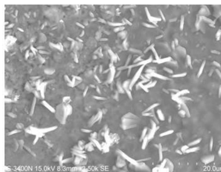
Fig(3b) Surface morphology of Mn doped ZnS thin films.
