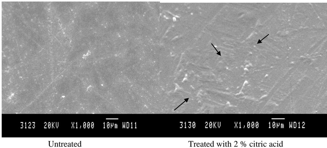
**Figure 3: Dual cross linked acrylic tooth specimen**
