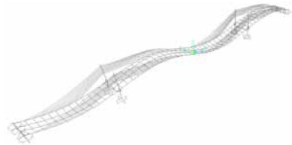
Figure 9: Mode 3 for span 48+120+48m, T=0.58s
