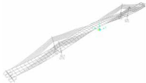
Figure 7: Mode 1 for span 48+120+48m, T=1.09s
