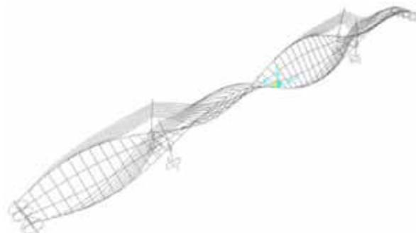
Figure 10: Mode 4 for span 48+120+48m, T=0.52s
