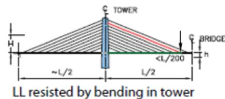
offset by dead load in main span; Short side span prevents backstay from going slack
