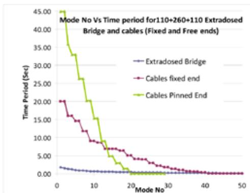
Figure13: Mode no Vs Time period (s) for structure and cables for 110+260+110m Extradosed bridge
