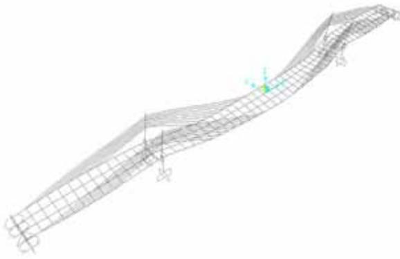
Figure 11: Mode 5 for span 48+120+48m, T=0.43s
