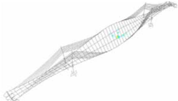
Figure 8: Mode 2 for span 48+120+48m, T=0.87s
