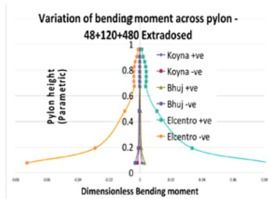
Figure 19: Variation of bending moment across pylon height for 48+120+48m span (Non-dimensionalized)
