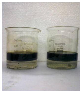
Photo graphs show esterification (biodiesel and residues layer), biodiesel production Fig 5.(a): Transesterification (b): Algal biodiesel
