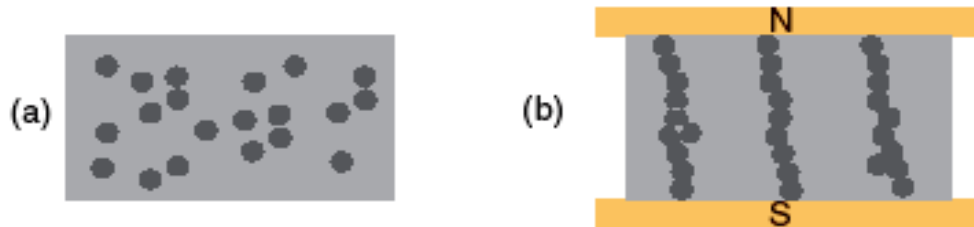
Fig. 1. Magnetorheological fluid: (a) no magnetic field and (b) with magnetic field
