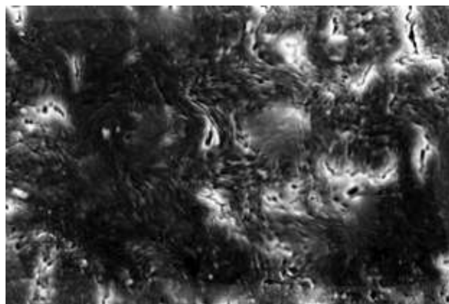
Fig 6: Scanning electron micrograph showing surface charring for CO 2 laser at 1.2 sec
