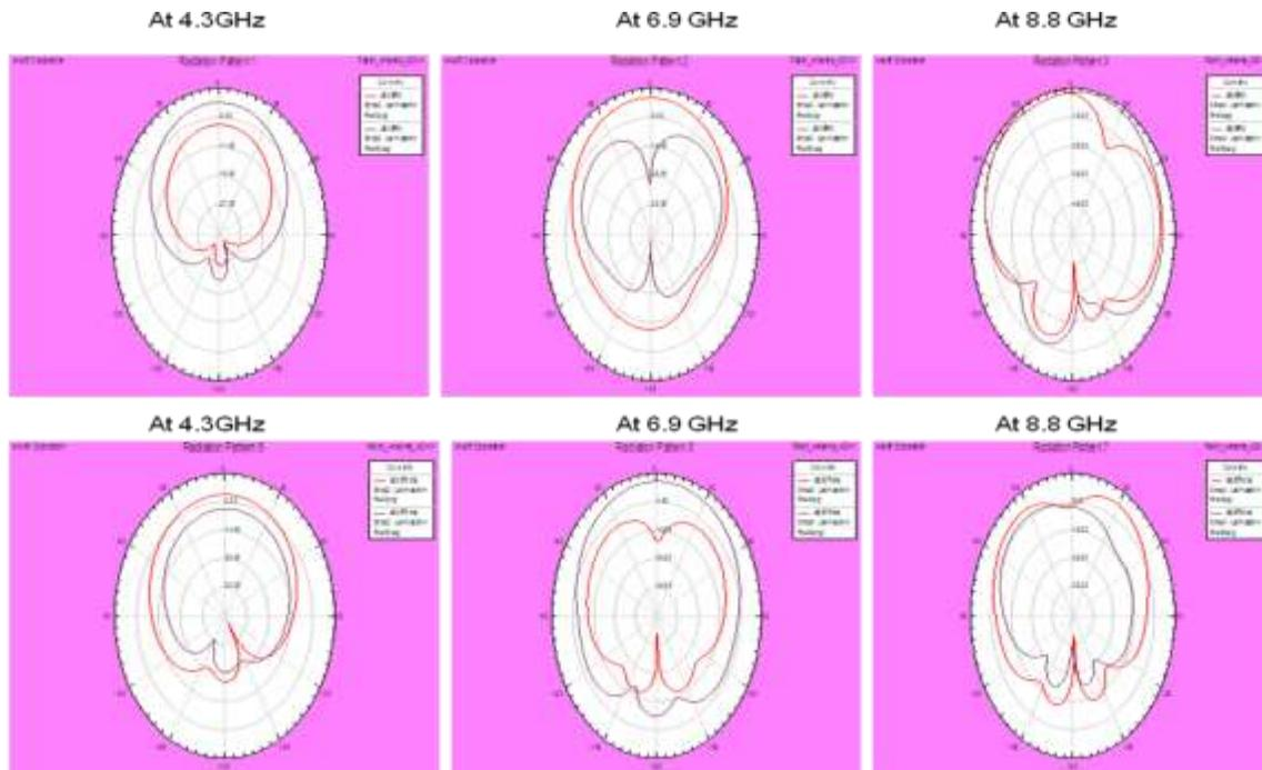
**Figure 5. Co-Polarization and Cross-Polarization radiation pattern of antenna at resonating frequencies**
