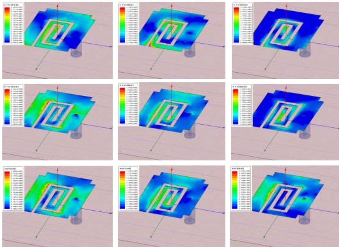
Figure 6. E-field, H-field and current distribution of antenna at three resonating frequencies
