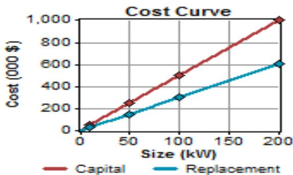
**Figure 7. Cost Curve of Wind Turbine (NW/100)**
