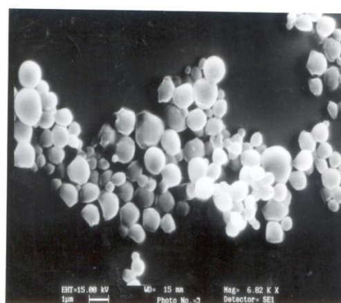
Figure: 2B - Scanning electron micrograph of microsphere preparation
