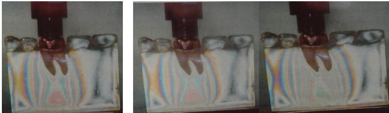
Figure 3: on vertical loading 30, 60,90 pounds
