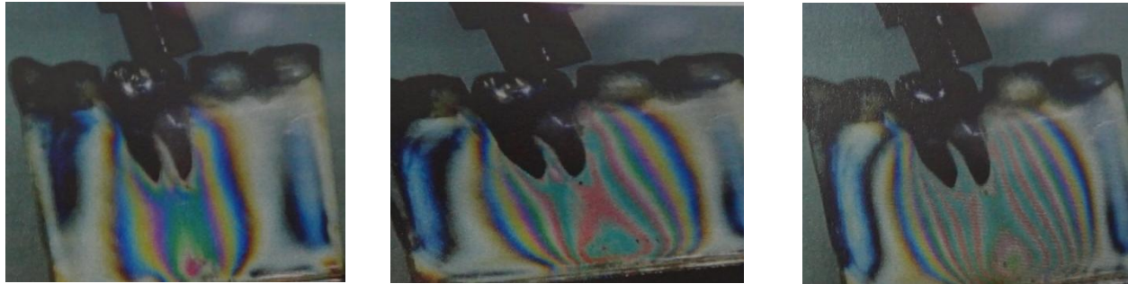
Figure : 6 On oblique loading Group III 30, 60, 90 pounds
