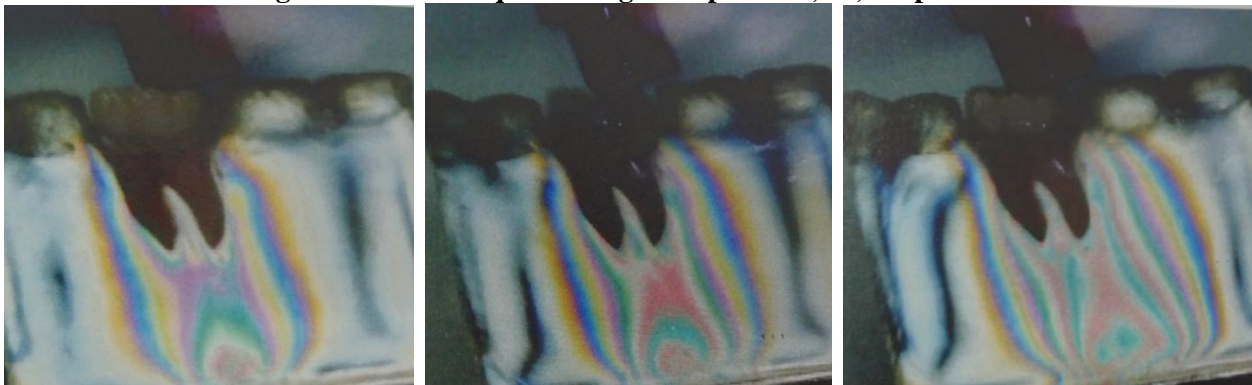
Figure : 10 On oblique loading Group VII 30, 60, 90 pounds
